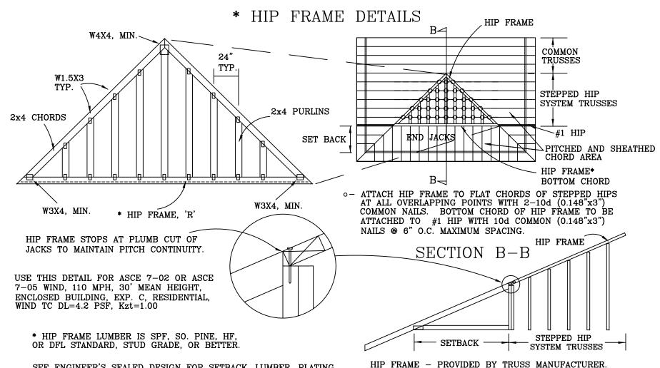
SEE ENGINEER'S SEALED DESIGN FOR SETBACK, LUMBER, PLATING, LOADING AND DURATION FACTOR REQUIRED.
